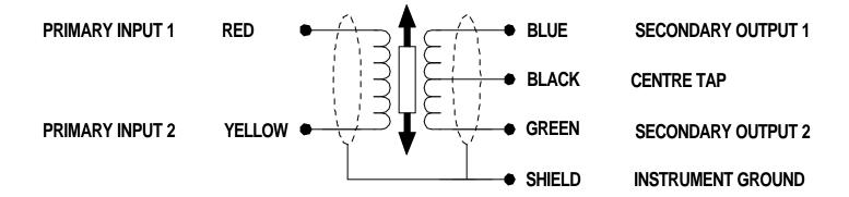
**Energising Supply:** 0.5 to 7V r.m.s. at 2 to 10kHz.
